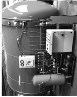
AIT AUTOCLAVE w/ COMPUTERIZED CONTROL PANEL
